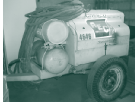
Air Compressor Two Stage Ingersoll Rand Model D-60 with air hammer
