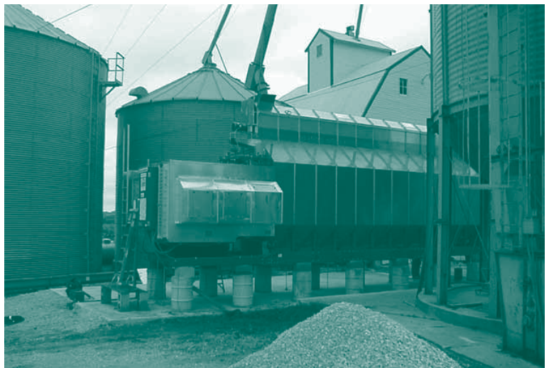
Replacement grain dryer installed on a Northeast Iowa farm.
