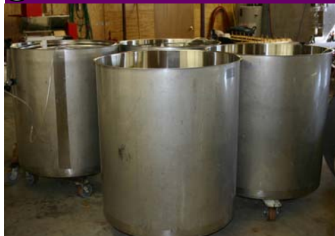
The juice is put in these steel vats and mixed with yeast and sugar and then stored for about 1-2 weeks.
