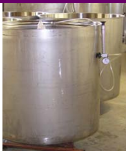
The next essential step is called "racking". Racking is the process of siphoning the wine off the sediments into a clean secondary fermentation container with a flexible plastic tube. This step is repeated 3-times.
