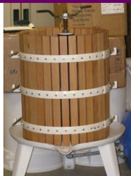
Then the grapes are placed in this 'press' to separate the juice.
