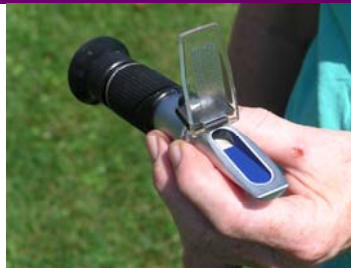
This essential tool, called a refractometer, helps determine when the grapes are ready. It measures the sweetness and acidity levels in terms of "brix".
