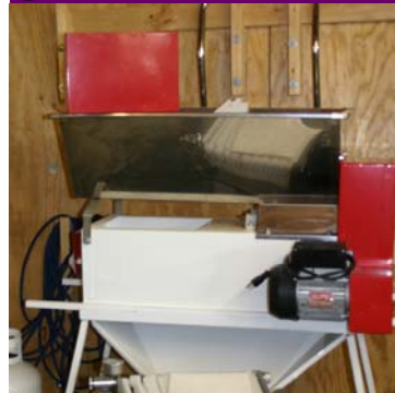
The grapes are placed in this machine which crushes and de-stems. The stems can cause a wine to taste bitter.
