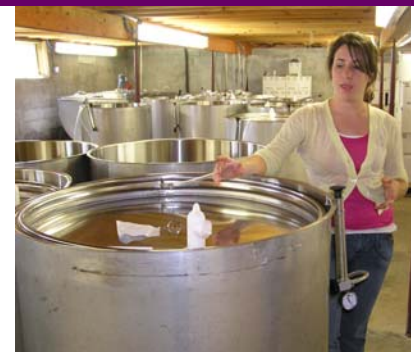
Nitrogen is injected into the steel vats to remove all oxygen. Air-tight lids are then secured and vats remain untouched for 6 months-1 year to allow the complete fermentation process.
